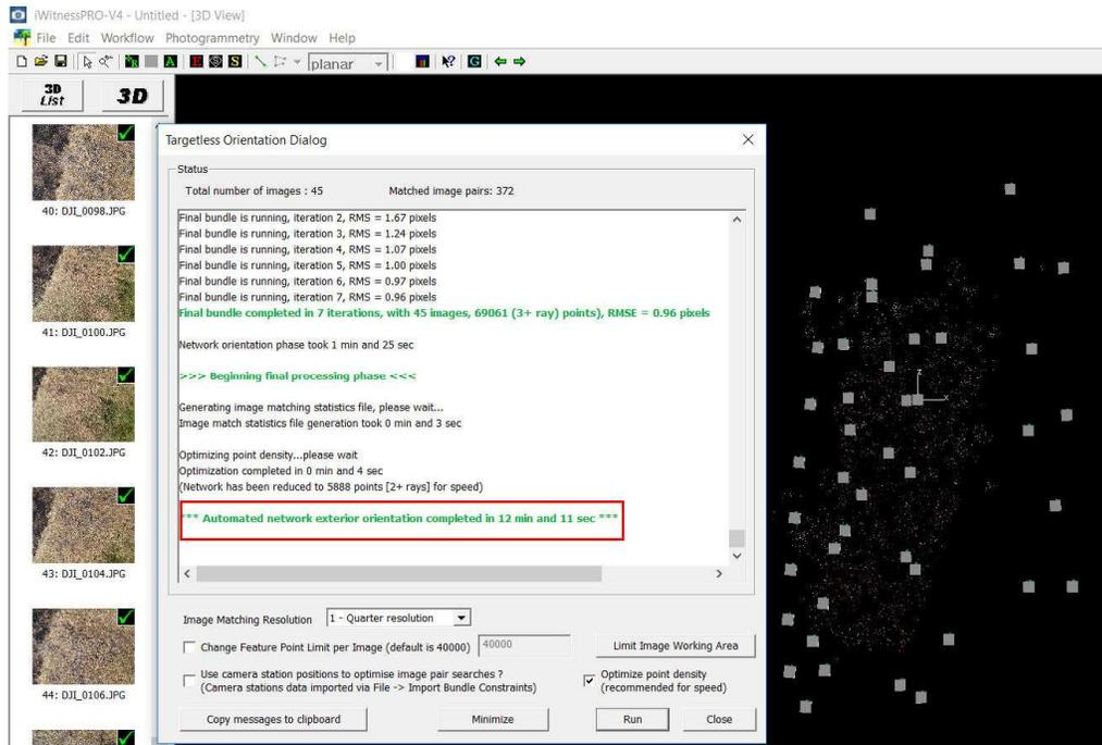
**Figure 1:** Output summary from iWitnessPRO network orientation and 3D point determination phase.
