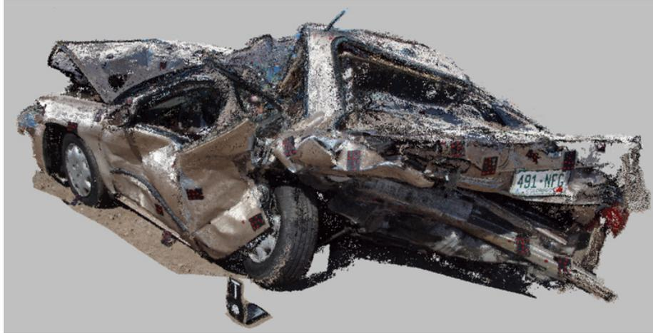
Figure 5: 3D model of crushed vehicle in the form of a dense point cloud.
