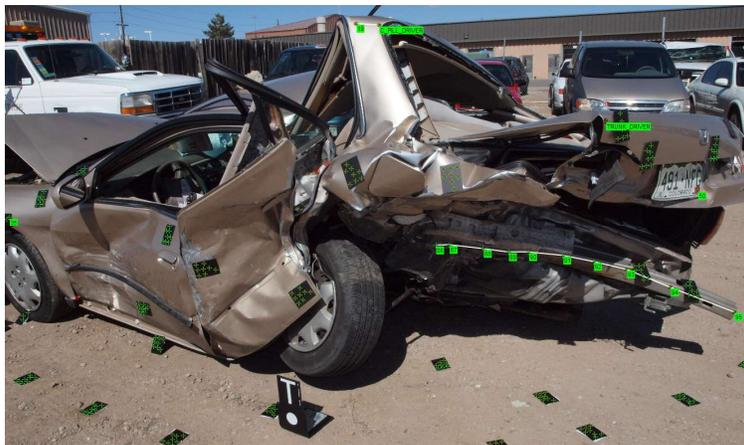
Figure 3: Image showing coded targets and feature points in the crush profiling
