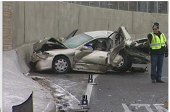
Figure 2: Vehicle to be crush profiled
