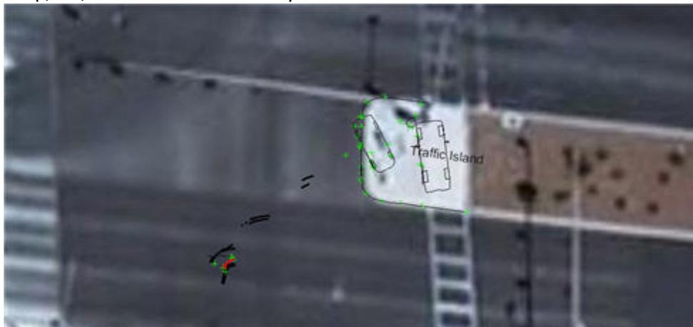
It took approximately one hour to “*iWitness* measure” the post-event images and also to rectify the single image in *XYRectify*. A further hour was required to complete the 3-image, 3D survey of the final vehicle rest positions using the trooper's Sony digital images, with the subsequent CAD diagramming also consuming about 1 hour.
