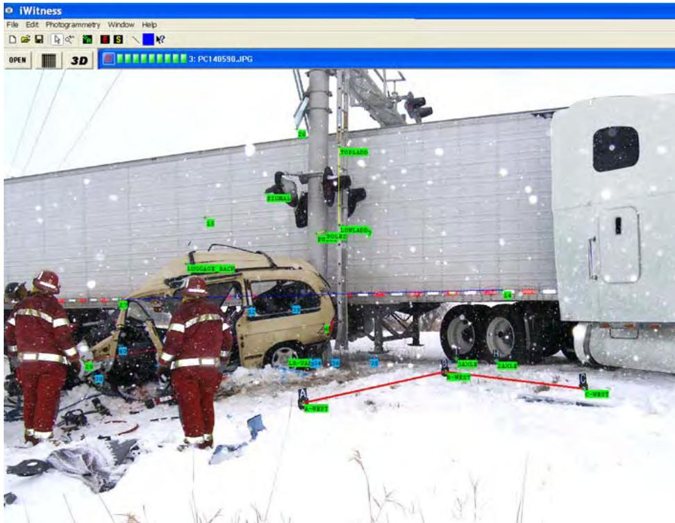
**One of nine digital images acquired by the Minnesota State Patrol and mapped using photogrammetry**
