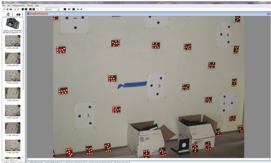
FIGURE 1 – Z-D calibration targets for DSLR and PAS cameras
